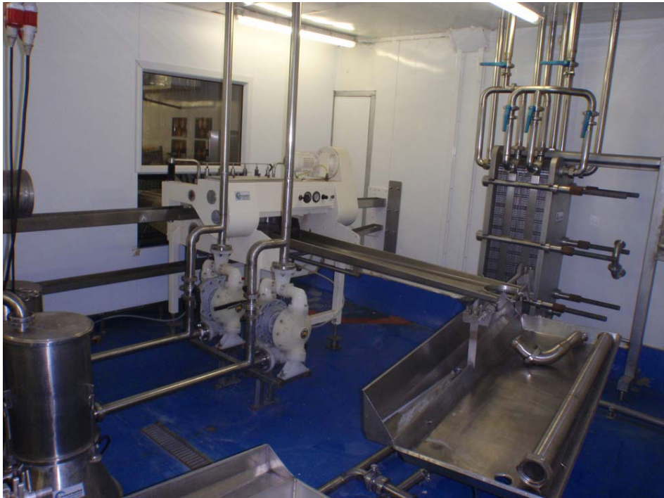
Separating system of the Egg Breaking Machine CEM 216
