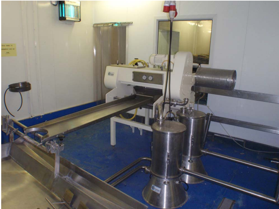
Separating system of the Egg Breaking Machine CEM 216
