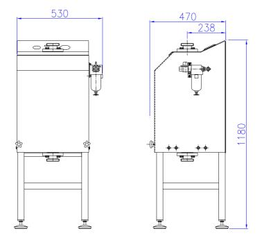
Capacity:15m³/hrAir consumption:5x product flow @ 6 bar (during C.I.P)
