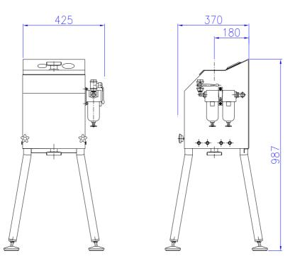
Capacity: Air consumption: 7*m<sup>3</sup>/hr* 5*x* product flow @ 6 bar (during C.I.P)
