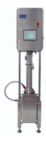
Coenraadts developed a new automatic filter with a special design (patented). It is a vertical automatic filter, which can be used in-line, with selfcleaning, and automatic evacuation of dirt during the operation and with minimal losses of product. This is achieved using a unique cleaning plunger in combination with a computerised control system.
